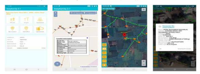
As shown in Fig 2, the same Mobile Application has additional functionality to utilize the point buffer analysis function of GIS development platform, by traversing the bus objects and terminal objects as listed under:
