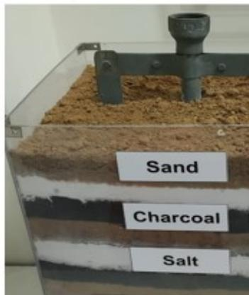
The installation of salt-charcoal type earthing is not done properly. They just mix up and fill up the pit. Even they use lesser depth of pit and mixture.
